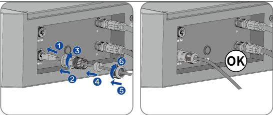
**Step5.** Connect the terminating resistor to the "Link Port Out" of the BCU.
