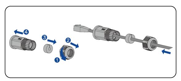
**Step4.** Connect the "Link Port In" of the BCU to the BMS port of the inverter using a shielded CAT 5 (or higher) ethernet cable. Tighten the cable gland and the insulator.
