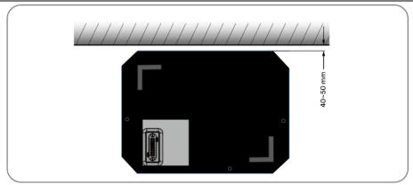
**Step3.** Remove a battery module from the package. Place one battery module on the base and secure the battery module with the supplied screws (M5×25, tightening torque 4 N·m). Pay attention to the direction of the module. The power connectors on the battery module and the base should be on the same side.
