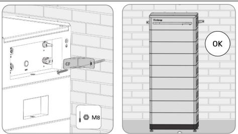
$\textbf{Step10.} Secure the hanger using screws (M8 \times 40).$
