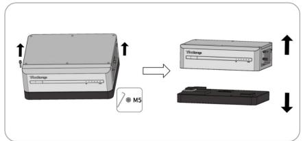
**Step2.** Place the base along the wall and ensure a distance of 40~50 mm between the wall and the base. Pay attention to the direction of the base. The power connectors on the base should be on the outside.
