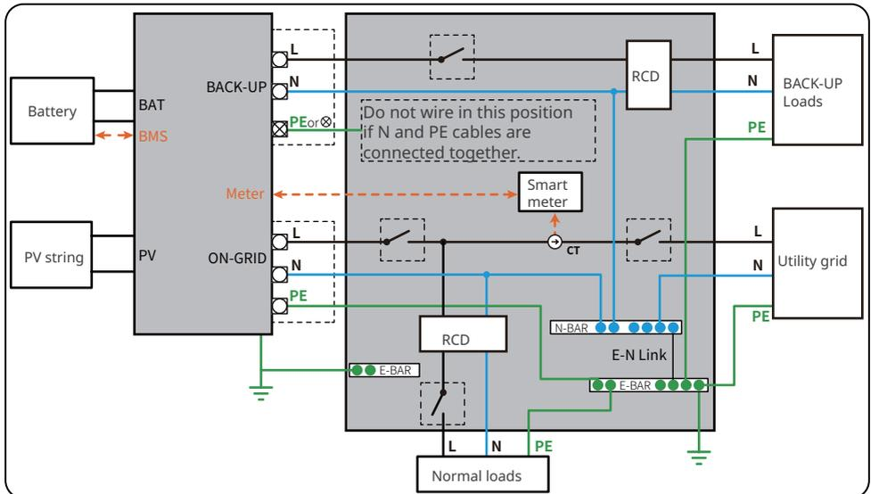
**N and PE cables are separately wired in the Main Panel.**
