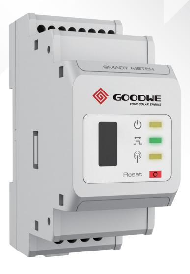
GoodWe Smart Meter is designed with high precision small dimensions, convenient operation and installation. It is available for both single-phase and three-phase grid system connection to detect voltage, current, power and energy, for working with inverters including SEMS systems for the purpose energy management.
